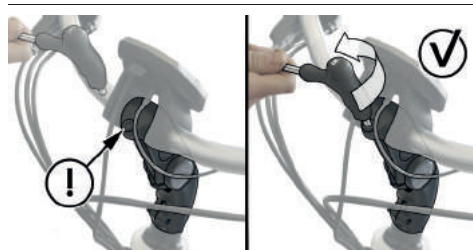
Image 9: Loosening the bolt on the stem
