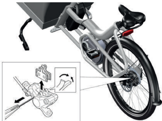
Image 38: Removing the brake pads in order to check them for wear
