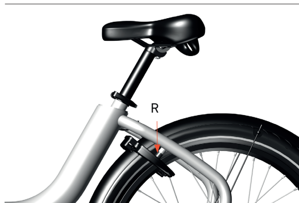
Image 37: Checking the lock rubbers
