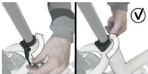
Image 8: Closing the seat post quick release
