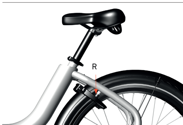
Image 37: Checking the lock rubbers
