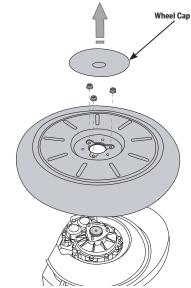
Figure 68: Remove the Tire/Wheel Assembly
