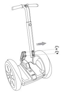
Figure 64: Remove LeanSteer Frame Fasteners
