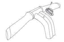
Figure 7: Install the InfoKey Controller Dock
