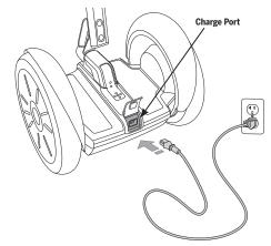
Figure 57: Plug Power Cord into Charge Port
