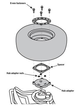
Figure 74: x2 SE Turf Tire/Wheel/Spacer/Hub Adapter
