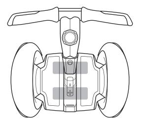
Figure 19: Controller Board Location
