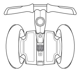
Figure 21: Balance Sensor Assembly Location
