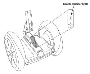
Figure 40: Balance Indicator Lights
