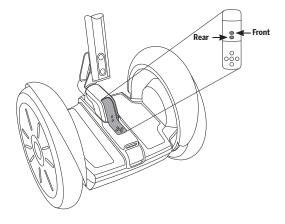
Figure 17: Battery Charge Indicator Lights
