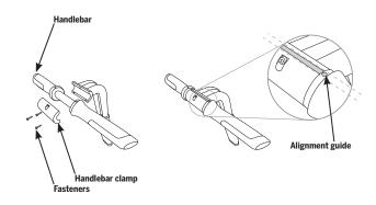
Figure 4: Attach the Handlebar
