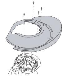
Figure 70: Remove/Install the Fenders
