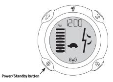
Figure 53: Powering Off The Segway PT
