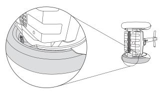
Figure 67: i2 SE Valve Stem Location
