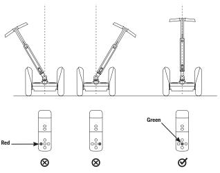
Figure 42: Ensure Balance Indicator is Green
