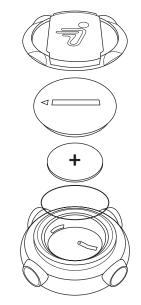
Figure 76: Replacing the InfoKey Controller Battery
