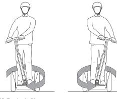
Figure 48: Turning In Place
