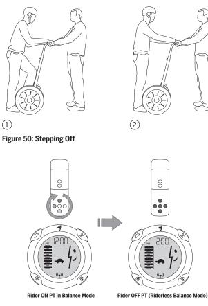
Figure 51: Transitioning to Riderless Balance Mode (Stepping Off)
