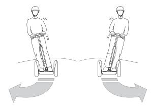
Figure 49: Turning While Moving
