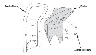
Figure 73: Remove the Fender from the Fender Frame
