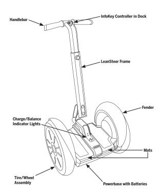
Figure 14: Segway PT Components
