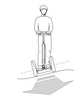
Figure 55: Keep the LeanSteer Frame Vertical on Slopes
