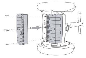
Figure 10: Torque the two center fasteners first.
