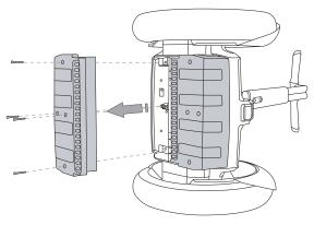
Figure 66: Remove the Batteries
