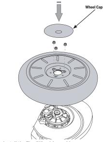
Figure 69: Install the Tire/Wheel Assembly
